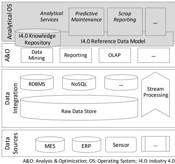
Figure 5: Concept of the analytical operating system
